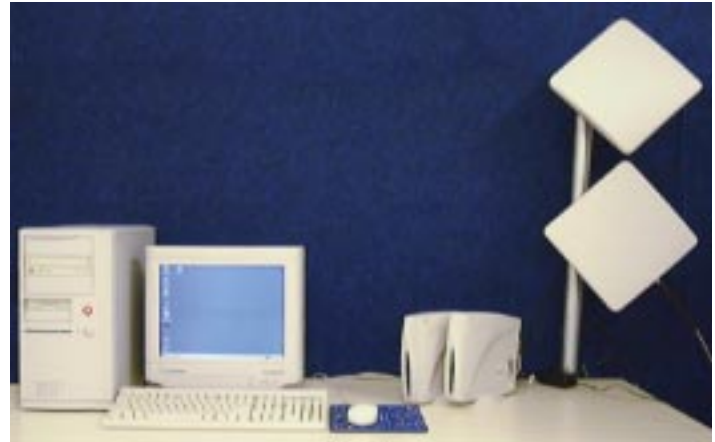
BWA-2003 subscriber equipment includes outdoor CPE Integrated Antenna/Transceiver (right) and indoor modem.
