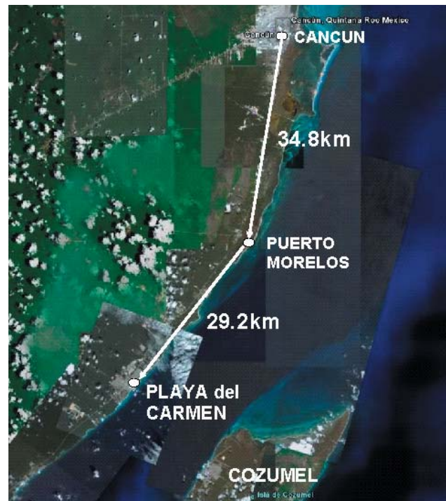
Two TVLINKS in series transport the broadcast TV signal from Cancun to Puerto Morelos and Playa del Carmen on Mexico’s Riviera Maya.
