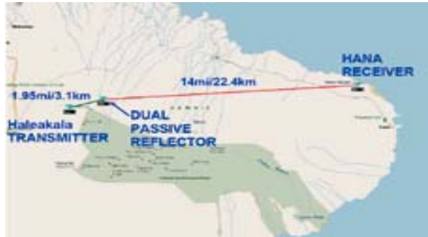
Link from Holoakala transmitter to Hanna (both in Maui, Hawaii) through a double passive reflector.
