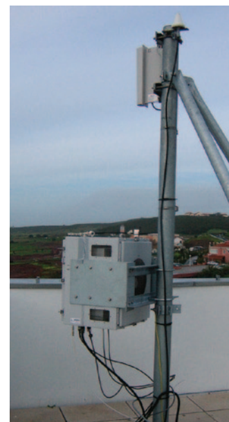
28 GHz high-power Base Station Transceiver integrated with 180-degree sector antenna.
