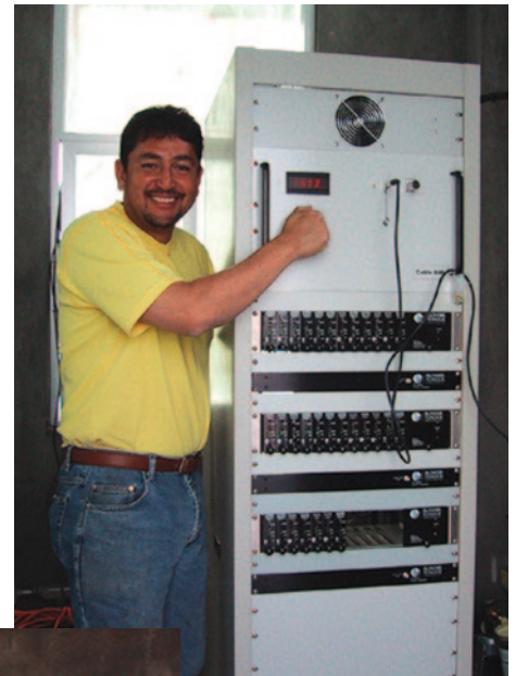
Armando Carrillo shows 250-Watt MMDS Transmitter integrated with compact headend.
