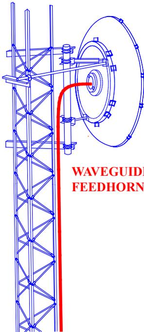
WAVEGUIDE FROM ANTENNA FEEDHORN TO RECEIVER INPUT
